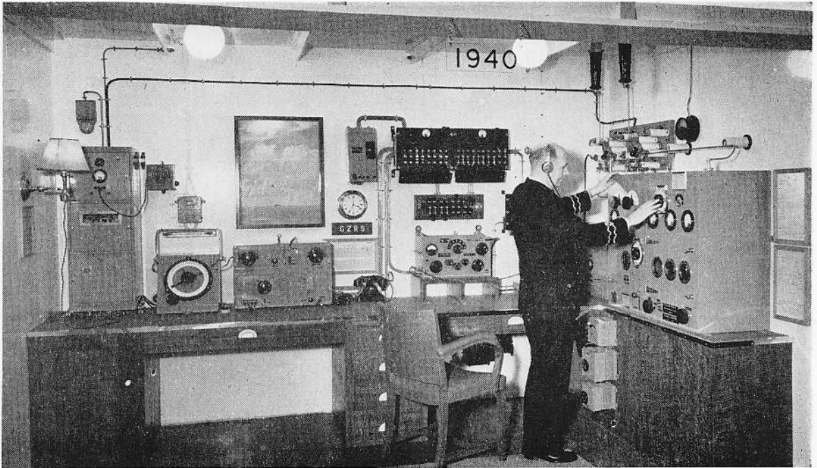
The short wave transmitter shown in this cabin brought about a tremendous increase in the range of communications and the Direction Finder equipment developed in earlier years, together with the Auto-Alarm embodying many new refinements
